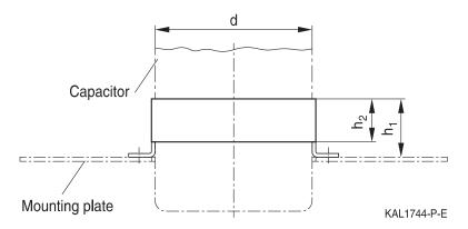
It is recommended to insert an additional insulating strip between capacitor and ring clip to avoid any risk of damage due to edges from the clip. The strip is included in delivery. For ordering code, see the following table. Attention must be paid to any relevant regulations (e.g. VDE, BSA or UL).
