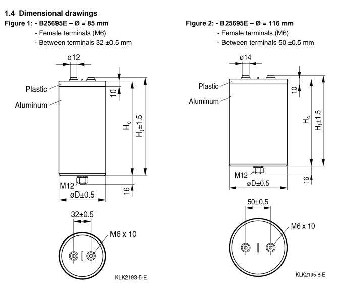
M12 stud on bottom of the aluminum case, nut (DIN 934) and toothed lock washer (DIN 6797) for fixing are standard for all types.
